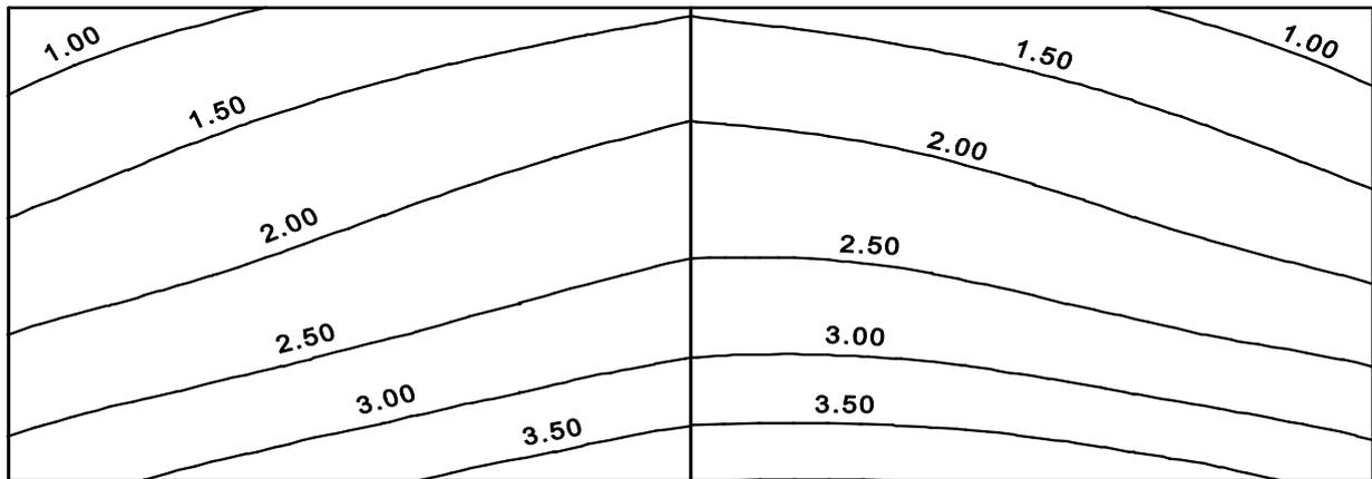
**Figure 4.63** Contour lines of settlements  $s$  [cm]
